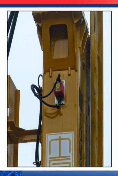
The **INCLINOCAN-2** bus unit is attached to the drill mast. It contains the X and Y inclinometers that measure the angles of the drill mast for positioning before drilling.
