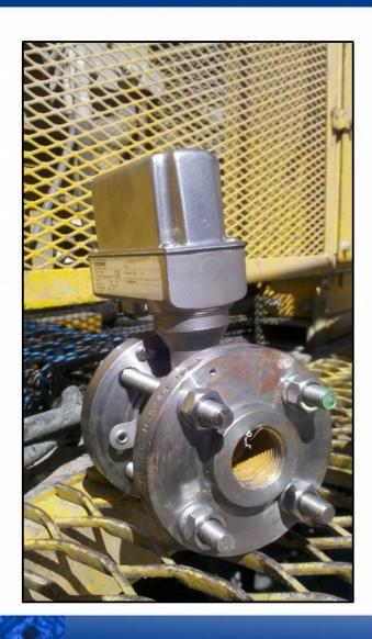
Installation of an electromagnetic flowmeter.
