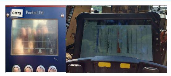
Repetition in real time of drilling parameters graphs displayed by PocketLIM to an external tablet.
